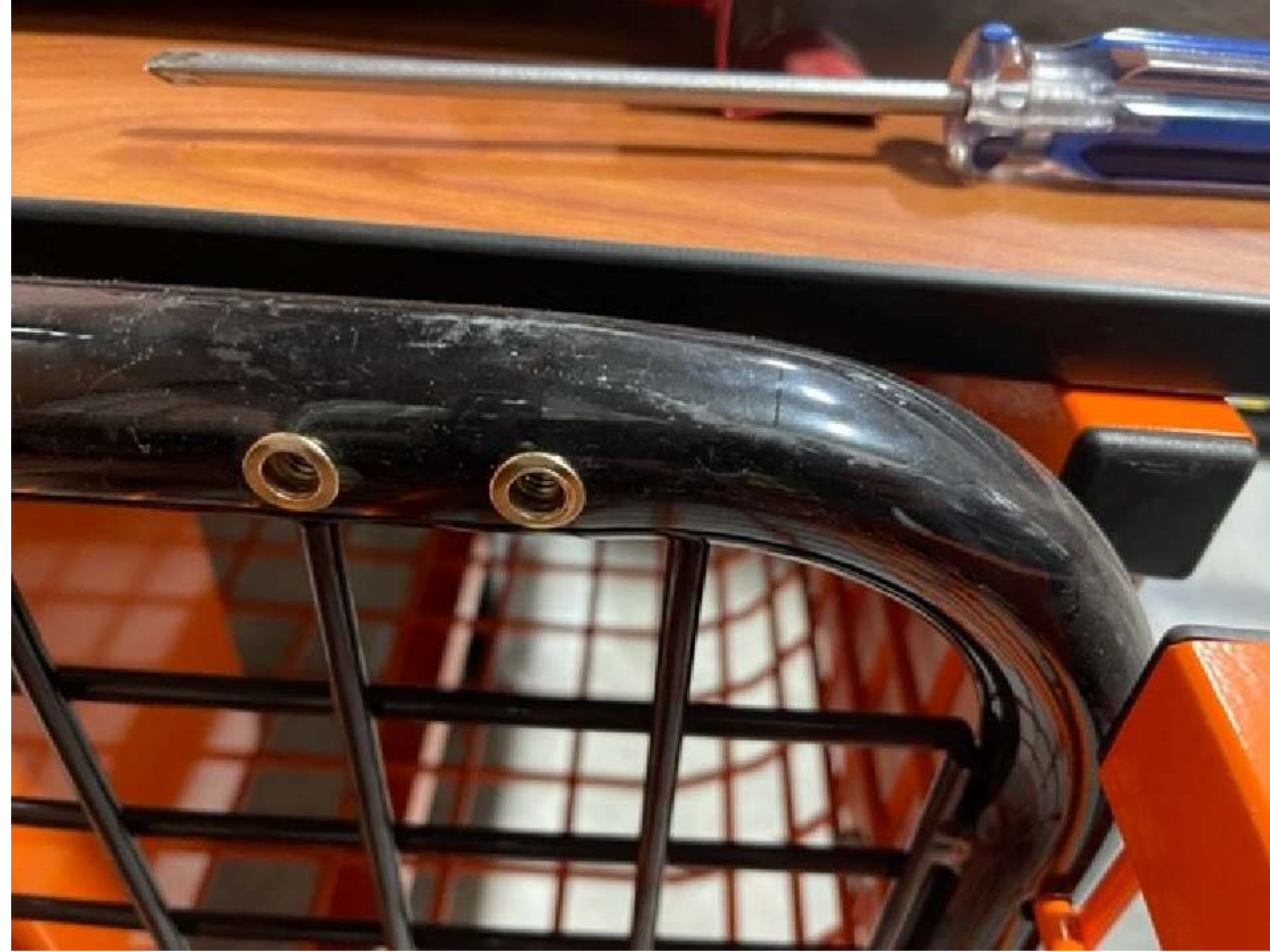
STEP 2 LOCATE THREADED NUTSERTS AS SHOWN ABOVE.
