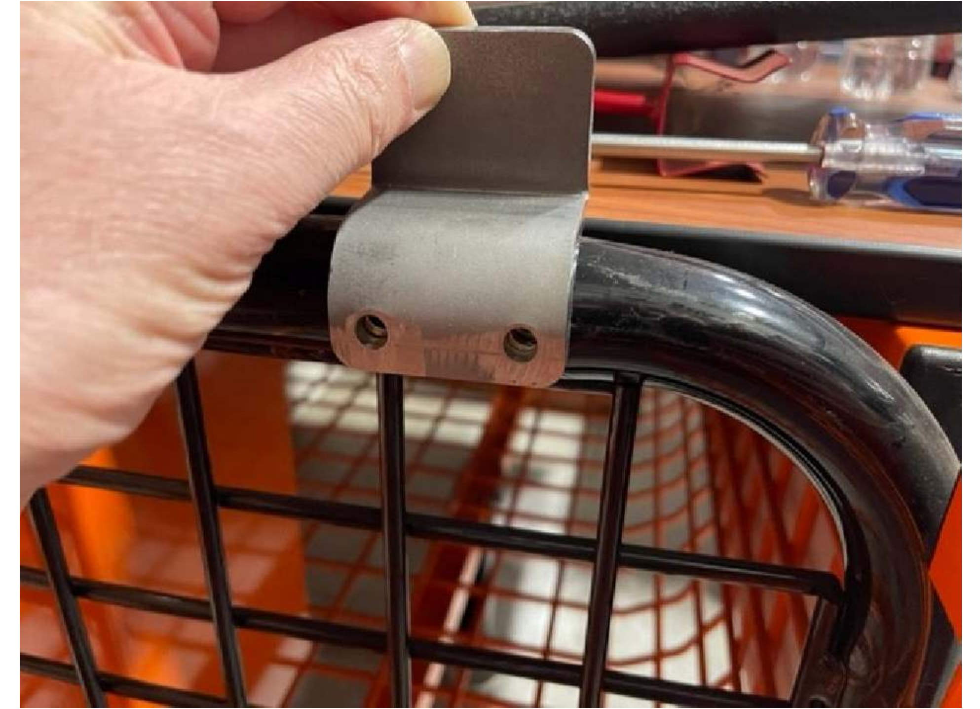
STEP 3 LINE UP DOOR STOP MOUNTING HOLES WITH THE THREADED NUTSERTS AS SHOWN.
